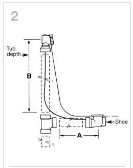
Install using ABS 1½" Schedule 40 DWV pipe in compliance with ASTM D  $\,$  2665-89a  $\,$  CONLY.
