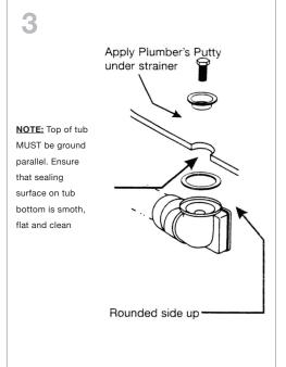
Mount Drain to tub with supplied drain screw.
