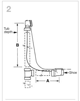
Install using PVC 1½" Schedule 40 DWV pipe in compliance with ASTM D  $\,$  2665-89a  $\,$  ONLY.
