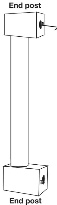
Install end posts on bar and tighten set screw securely.
