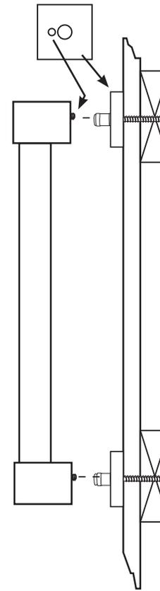
Install grab bar onto mounting flange post on wall. Be sure square escutcheons are straight and that set screw on base of end posts are installed and line up with one of the two holes in the escutcheons.
