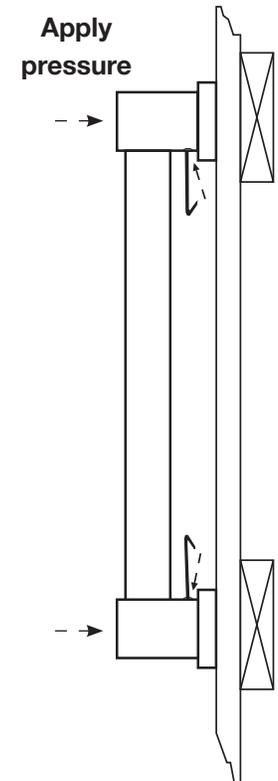
Using allen wrench, tighten set screws while applying pressure to end posts.
