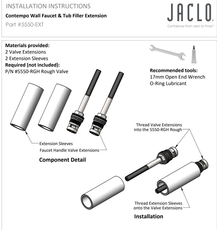
**Step 1:** Apply suitable lubricant to the Faucet Handle Valve Extension O-rings.
