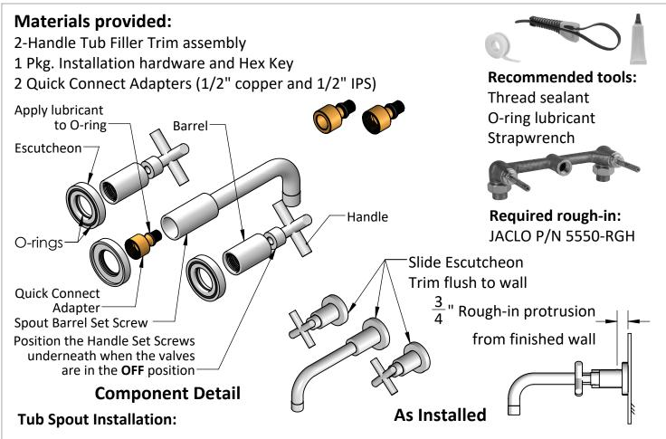
**Step 1:** Determine if the existing rough-in is either a 1/2" IPS or 1/2" copper sweat. The Spout rough-in pipe should protrude from the finished wall 3/4".
