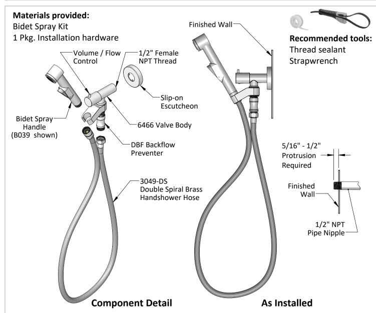
**Note:** These kits are equipped with a built-in positive shut-off valve. Any of JACLO's pressure balance valves or JACLO's 1/2" thermostatic valves with built-in volume controls can be used as the primary positive shut-off and mixing valve for temperature control.
