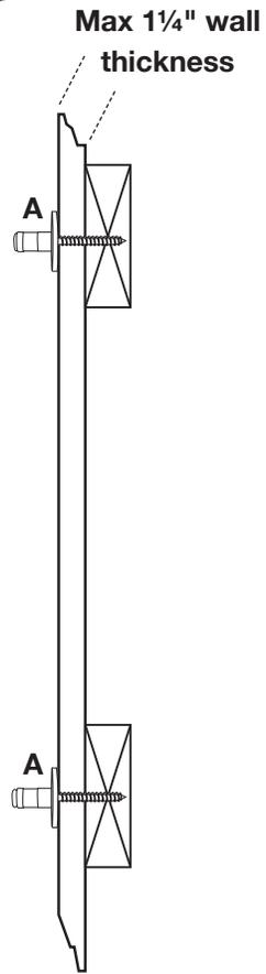
Determine bar position. Place mounting flange **(A)** on wall. Drive #14 x 3" screw into 1" plywood or wood stud. Tighten completely.
