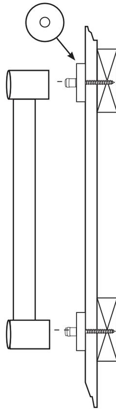
Install grab bar onto mounting flange post on wall.
