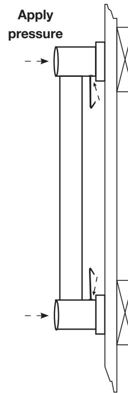
Using allen wrench, tighten set screws while applying pressure to end posts.
