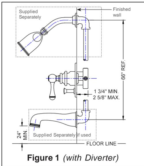
**Figure 1 (with Diverter)**
